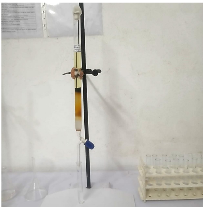
Figure 1: Isolation of components by column chromatography.
