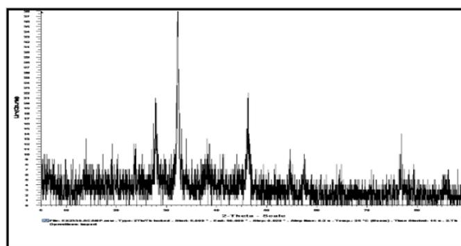
**Figure 4:** XRD analysis of SASNPs.
