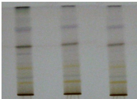
Figure 5: HPTLC MEAL fingerprint profile at visible region, where T1, T2 and T3 are the concentrations of 1 mg/mL solution in methanol developed on a silica gel G60 F 254 plate in triplicates that were eluted with Toluene: Ethyl acetate: Methanol: Glacial acetic acid (55: 35: 10: 2) as the mobile phase.
