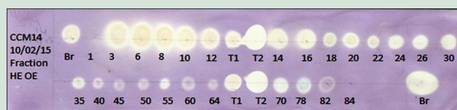
Figure 2: Image of the silica plate with the essential oil fractions of Origanum elongatum after 15 min reaction with DPPH. DPPH at 6 \cdot 10^{-5} M. Br: Crude essential oil, 1-84: Selected fractions. T1: \delta -tocopherol; T2: Ascorbic acid. DPPH: 2,2-diphenyl-1-picrylhydrazyl
