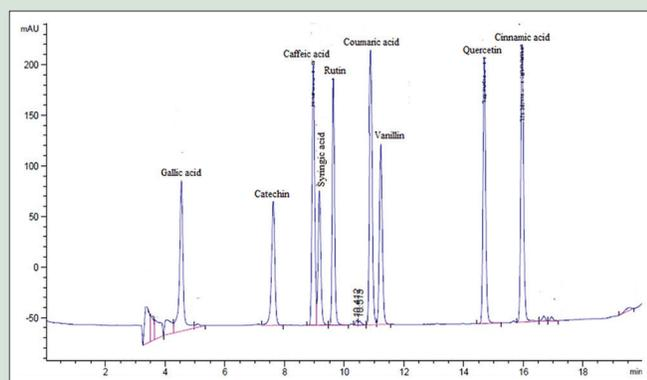
**Figure 2:** High performance liquid chromatography chromatogram of nine standard phenolic compounds; gallic acid (1), catechin (2), caffeic acid (3), syringic acid (4), rutin (5), coumaric acid (6), vanillin (7), quercetin (8), and cinnamic acid (9)
