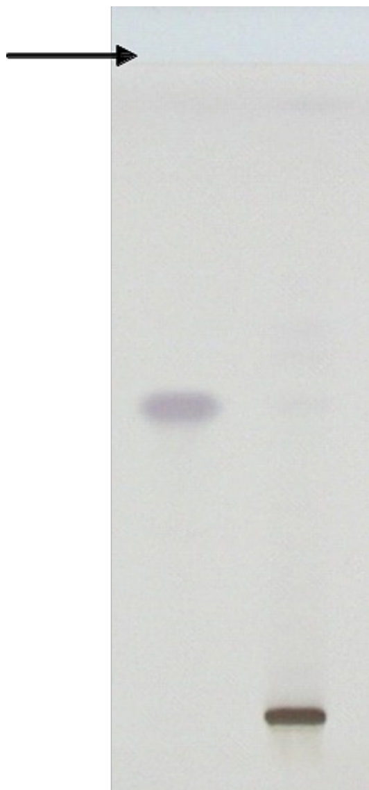
Figure 3: HPTLC profile of C. macleodii bark under 600 nm along with \beta -Sitosterol (STD).
