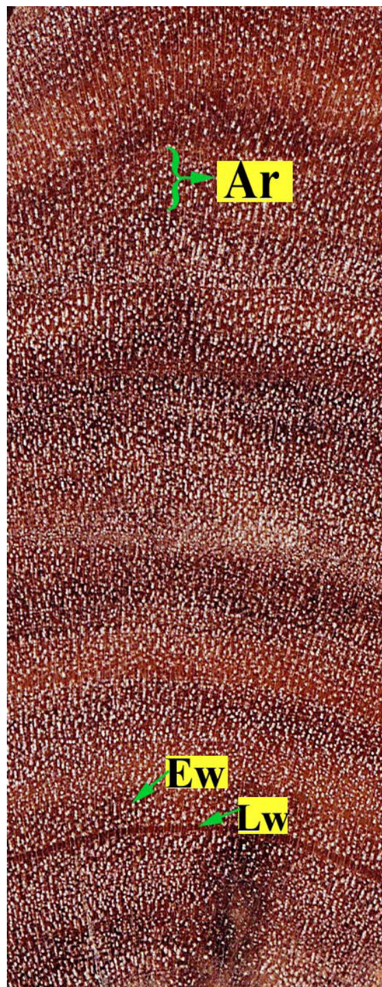
Figure 3: Macro-morphology of transversely cut heartwood.
